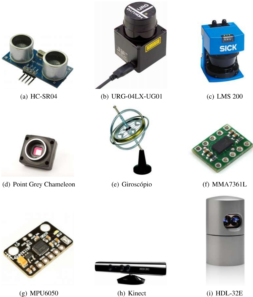
Figura 6.2. Exemplo de sensores: (a) sonar HC-SR04 [Cytron Technologies 2015], os sensores laser (b) URG-04LX-UG01 [Hokuyo Automatic 2015] e (c) LMS 200 [SICK 2015], (d) câmera Point Grey Chameleon [Point Grey Research 2015], (e) Giroscópio mecânico, (f) acelerômetro MMA7361L [Freescale Semiconductor 2015], (g) IMU MPU6050 [InvenSense 2015], (h) Microsoft Kinect e (i) Velodyne HDL-32E [Velodyne LiDAR 2015].
