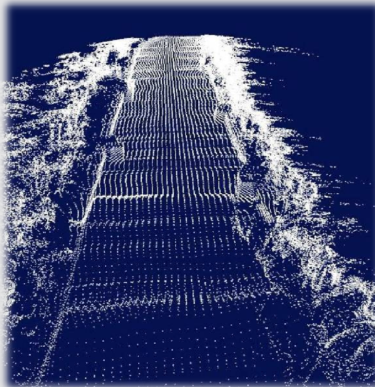
3D environment map: used to detect obstacles and road imperfections
