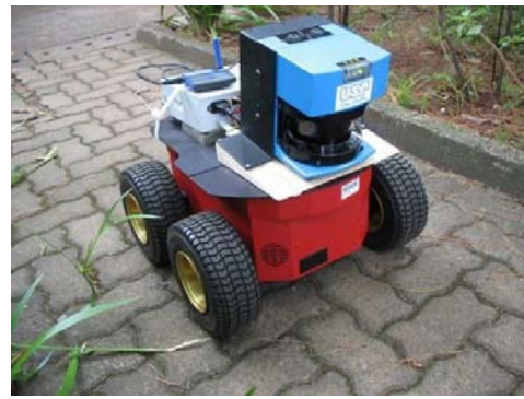
Figure 1: Pioneer AT Robot used in the experiments.
