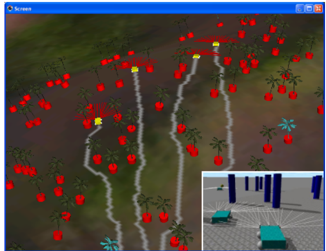
Figure 4. Detailed view of navigation with obstacles avoidance.
