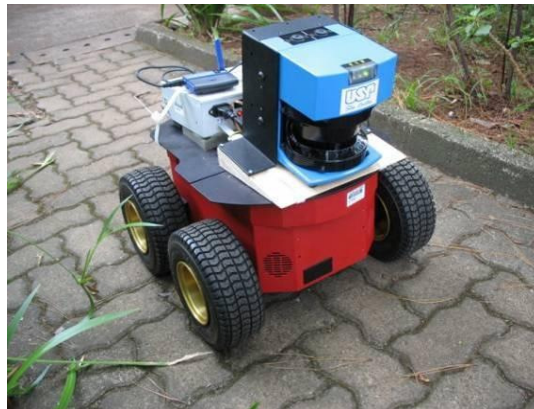
Figure 1. Pioneer 3 AT Robot and SICK LMS 200 LRF used in the experiments.
