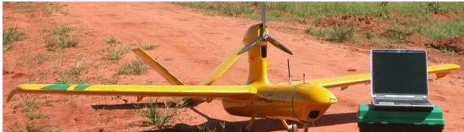
Fig. 9. ARARA Project under development at LRM Lab: Autonomous UAV capable of following a pre-defined GPS way-point
