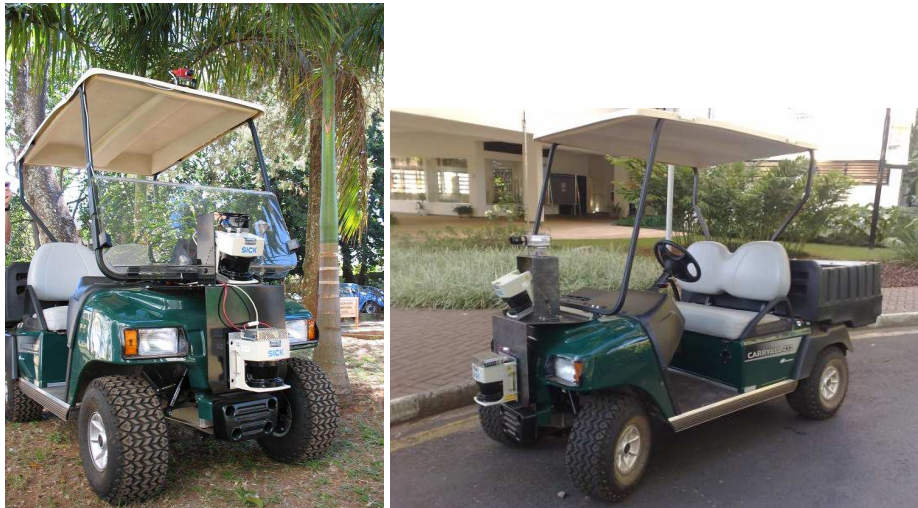
Fig. 8. Electrical Autonomous Vehicle under development at LRM Lab: Club Car equipped with Roboteq Motor Controller (Steering), Laser Sick and Camera
