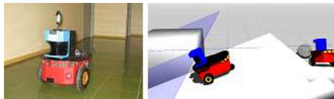
Fig. 6. Pioneer DX robots: real and simulated
