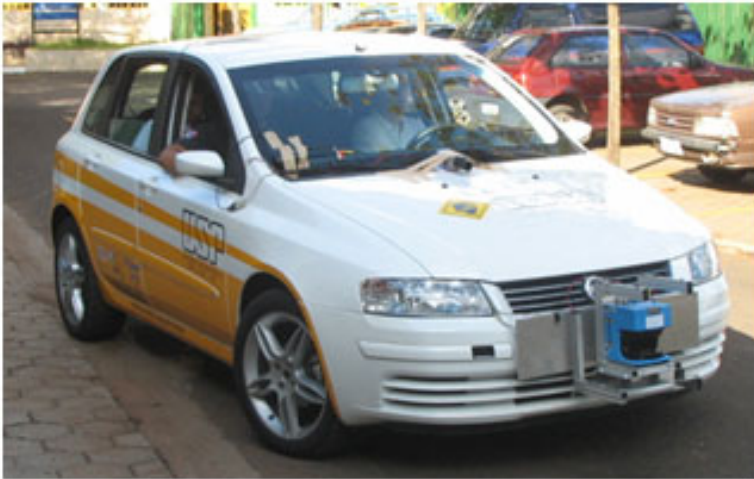
Fig. 2. Vehicle used in experiments equipped with a frontal Sick LMS 200 Laser sensor and with a compass and GPS system
