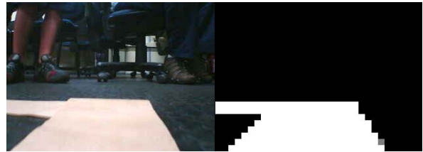
Fig 10 – Comparison between a 90 ° left turn frame and the navigability map generated from it
