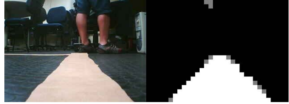
Fig 9 – Comparison between a straight way frame and the navigability map generated from it
