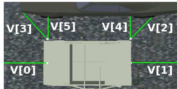
Figure 1. Distribution of the sonar sensors
