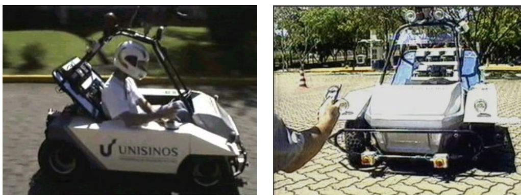
Figura 4.31: Mini-Baja com Tecnologia drive-by-wire
