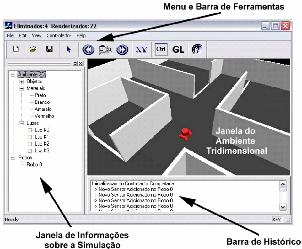
Figura 4.21: SimRob3D – Interface do Simulador
