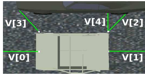
Fig. 4. Distribution of the sonar sensors around the vehicle
