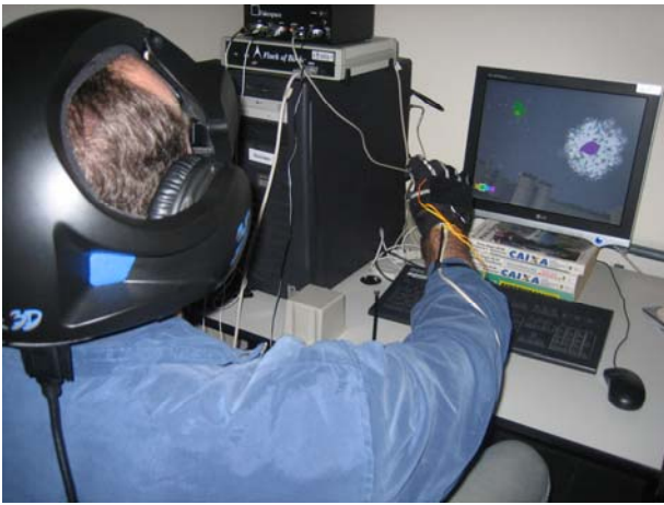
Figure 5. User playing GhostHunt with the proposed technique: he is wearing a head-mounted display, a pinch glove and a 3D tracker on his arm.
