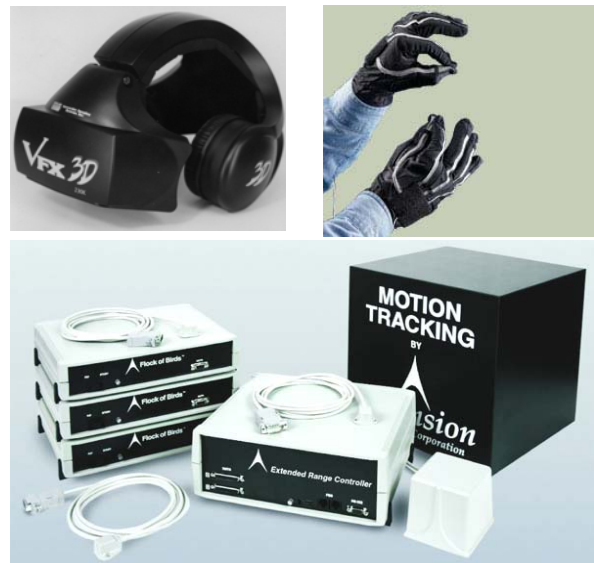
Figure 3. Devices used. Top-left: VFX3D (head-mounted display). Top-right: Pinch Gloves (data glove). Bottom: Flock of Birds (3D tracker).
