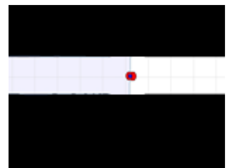
a) Robot in a corridor with corresponding laser scan area (in blue)
