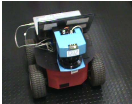
Fig. 8. Pioneer P3-AT robot with Sick Lidar used in experiments
