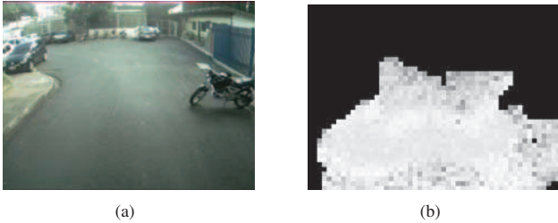
Fig. 6. (a) is a color image. (b) is results from a classification sample from our system. Black represents non-road class, white represents road class and the gray represents the intermediate values.
