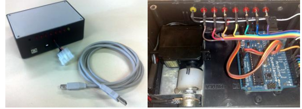
Fig. 3. Throttle controller device. At right, the inside view with highlights to Arduino and mechanical coupling between servo motor and potentiometer.
