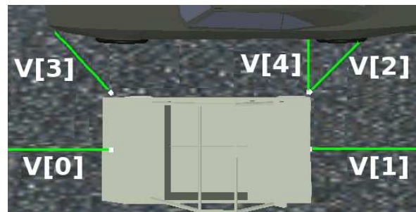
Figure 4: Distribution of the sonar sensors around the vehicle
